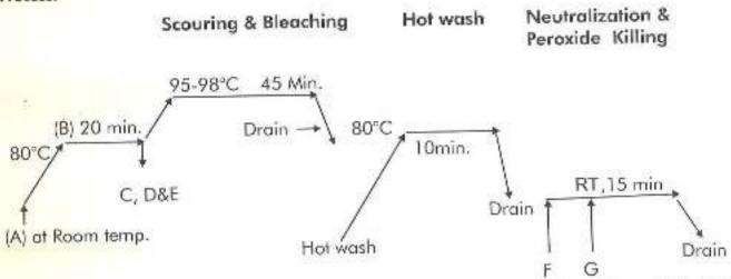
Charge Sebwet CP - 0.3% (A) at room temperature. Raise temperature to 60°C and dose Addiscour PCLP - 0.8% (B). Maintain temperature for 20 minutes. Charge Sebaux WDS - 0.25% (C), Hydrogen Peroxide — 1.5% (D) & Soda Ash - 1% (E). Raise temperature to 95°C, Boil for 45 min, Drain, Hot wash, Acetic Acid (F), Addisc 101 (G) Neutralization & Peroxide Killing
